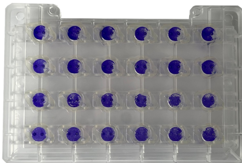
Figure 2. Cells attached in every well of the sensor plate stained with CV and dried overnight.
